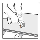
**3. Secure with screws** Secure with 2 x 50mm NoMorePly Fibre Cement screws per joist. Ensure screws are placed a minimum distance of 25mm from the tongue and groove edge.
