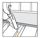
2. Stick boards to joists TG4 Tile Backer can be fixed to timber or steel joists installed at maximum 600mm centres using 22mm and 450mm centres using 18mm. Apply a bead of Slow Set Mega Strength PU Adhesive to the joist, then position the first board. The foil tubes are better for larger areas.
