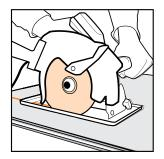
1. Cut boards to size Cut TG4 Tile Backer using a circular saw fixed with a vacuum extractor and a PCD Saw Blade. When cutting always use vacuum extraction with a suitable filter. This method will cut boards easily and reduce dust. Boards are fixed with board text facing up.
